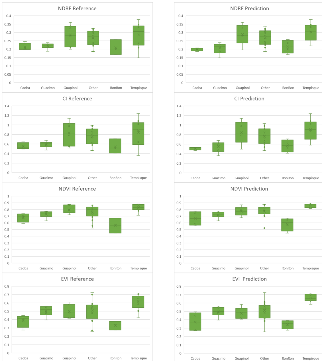
Figure 16: Box-Plots of reference (left) and prediction (right) derived VIs. Normalized Difference Red Edge Index (NDRE), Red-Edge Chlorophyll Index (CI), Normalized Difference Vegetation Index (NDVI) and Enhanced Vegetation Index (EVI) are displayed.
