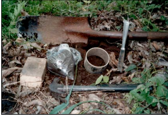
Figure 7-6: Sampling cylinder and implements of the sampling.
